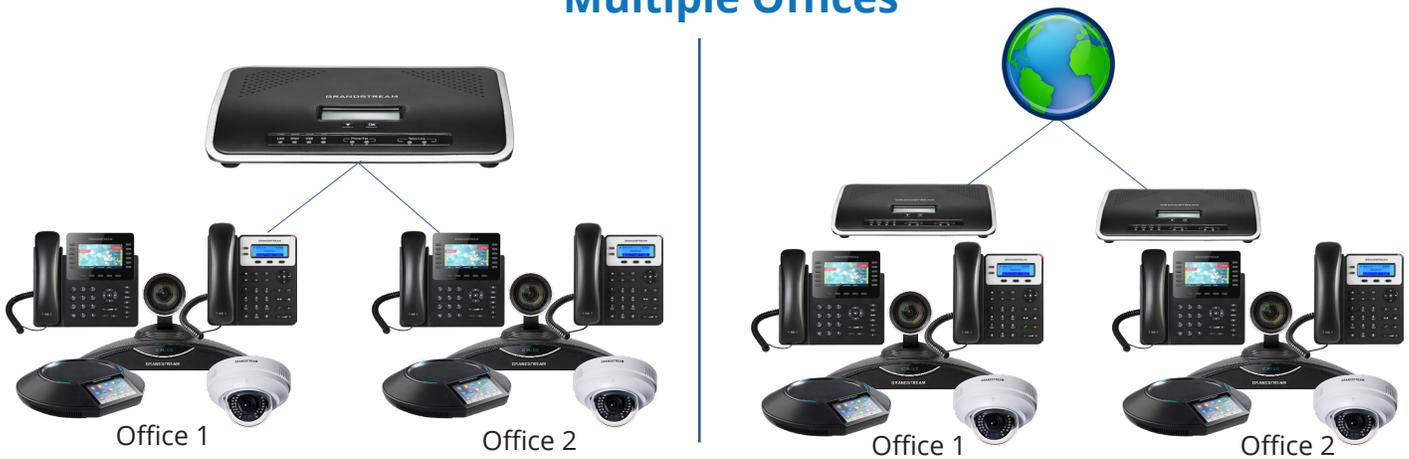
For business with multiple locations, multiple UCMs can be peered together, or a centralized UCM can support multiple locations. Peering allows all employees to be on the same network no matter what office they are in, while also making installation and management as simple as possible.
