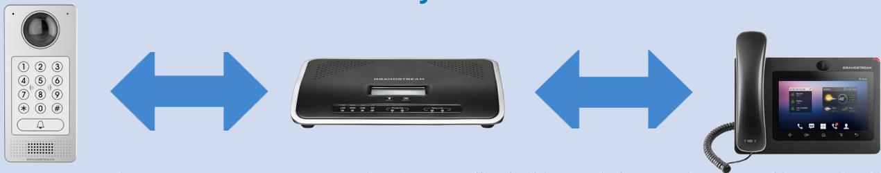
Put a door camera at the entrances to an apartment, dormitory or office building and place a video phone, like our GXV3275, in the apartments, dorm rooms or offices to allow visitors to be easily let in while also keeping the facility secure. The whole network is registered to and anchored by the UCM series IP PBX. .
