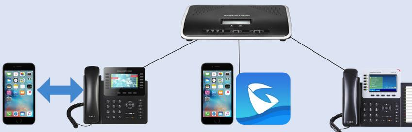
Support your remote employees and traveling workers with the UCM series by being able to support remote extensions, by using our free Grandstream Wave Softphone App on any Android or iOS device, or by having calls forwarded to any mobile phone number.
